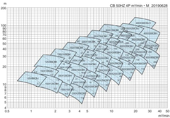
Note1 : The values inside the broken lines are motor output(kW) in case of density 1.0kg/L and viscosity 1.0mPa • s.
